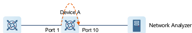
Figure 4-1 Port Mirroring Principles Figure
